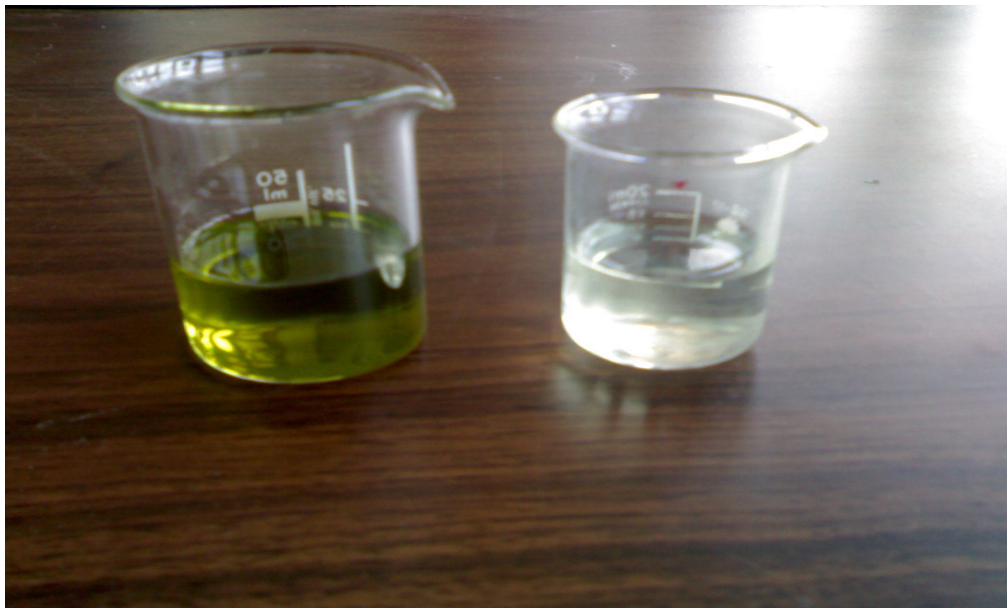
Fig. (3): Photograph showing the difference between the commercial phosphoric acid (to the left) and the obtained clear one.
