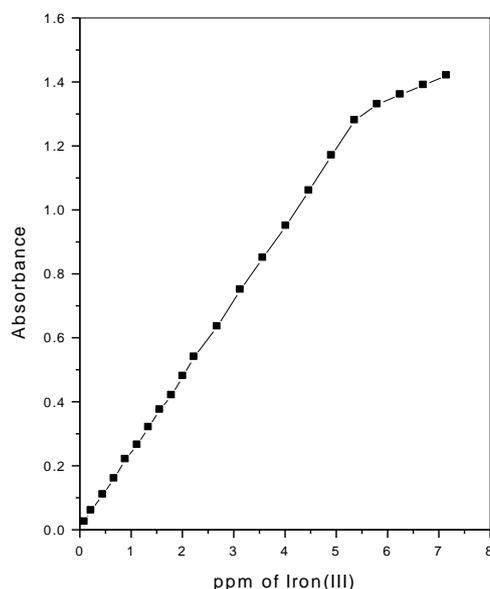
Fig.(4): Calibration graph for the determination of iron(III) with SHAM as binary complex.
