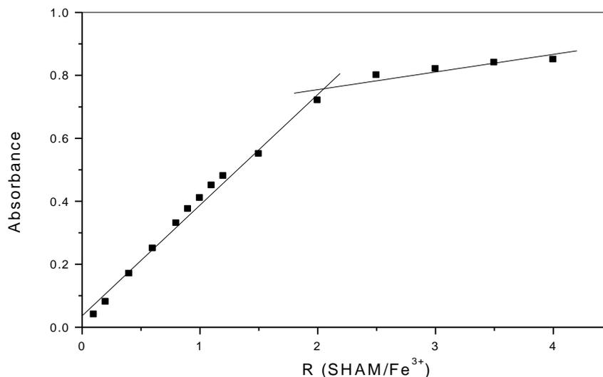
Fig.(5): Determination of iron(III)-SHAM ratio in the binary complex using the molar ratio method
