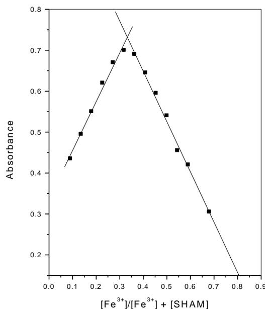
Fig.(6): Determination of iron-SHAM ratio in the binary complex using the continuous variation method.
