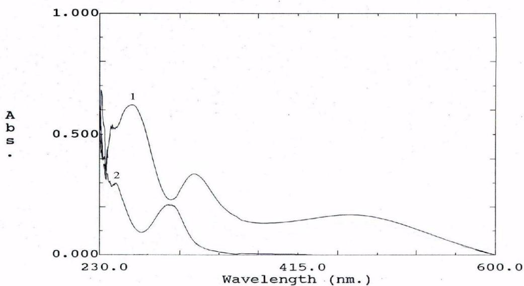
Fig.(2): Absorption spectra of iron(III)-SHAM complex. curve 1, the binary complex; curve 2, its reagent blank.
