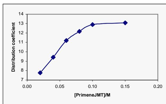
Fig.1 Effect of different concentrations of primene-JMT on the distribution coefficient of lanthanum
