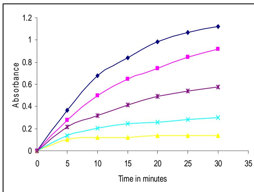
Figure 3: Absorbance versus time graph for the reaction between EN ( $5 - 40 \mu\text{g ml}^{-1}$ ) and potassium permanganate
