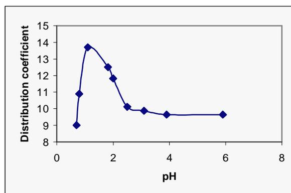
Fig.3 Effect of pH on the distribution coefficient of lanthanum.
