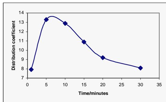
Fig.2 Effect of contact time on the distribution coefficient of lanthanum
