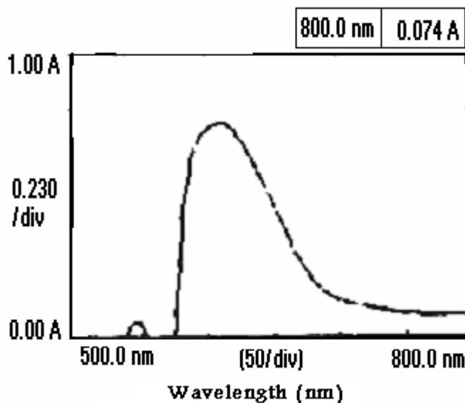
Figure 2: absorption spectrum of manganate ion obtained after the reaction of  $\text{KMnO}_4$  with FOS ( $50 \mu\text{g ml}^{-1}$ ).
