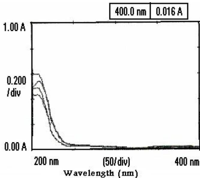
Figure 1: Absorbance spectra of EN( $25 \mu\text{g ml}^{-1}$ ), RM( $25 \mu\text{g ml}^{-1}$ ), LS( $25 \mu\text{g ml}^{-1}$ ) and FOS( $25 \mu\text{g ml}^{-1}$ ) in water
