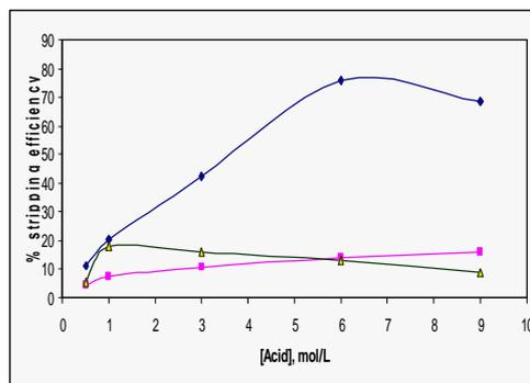
Fig. 4 Effect of different acidic stripping agents on stripping process
