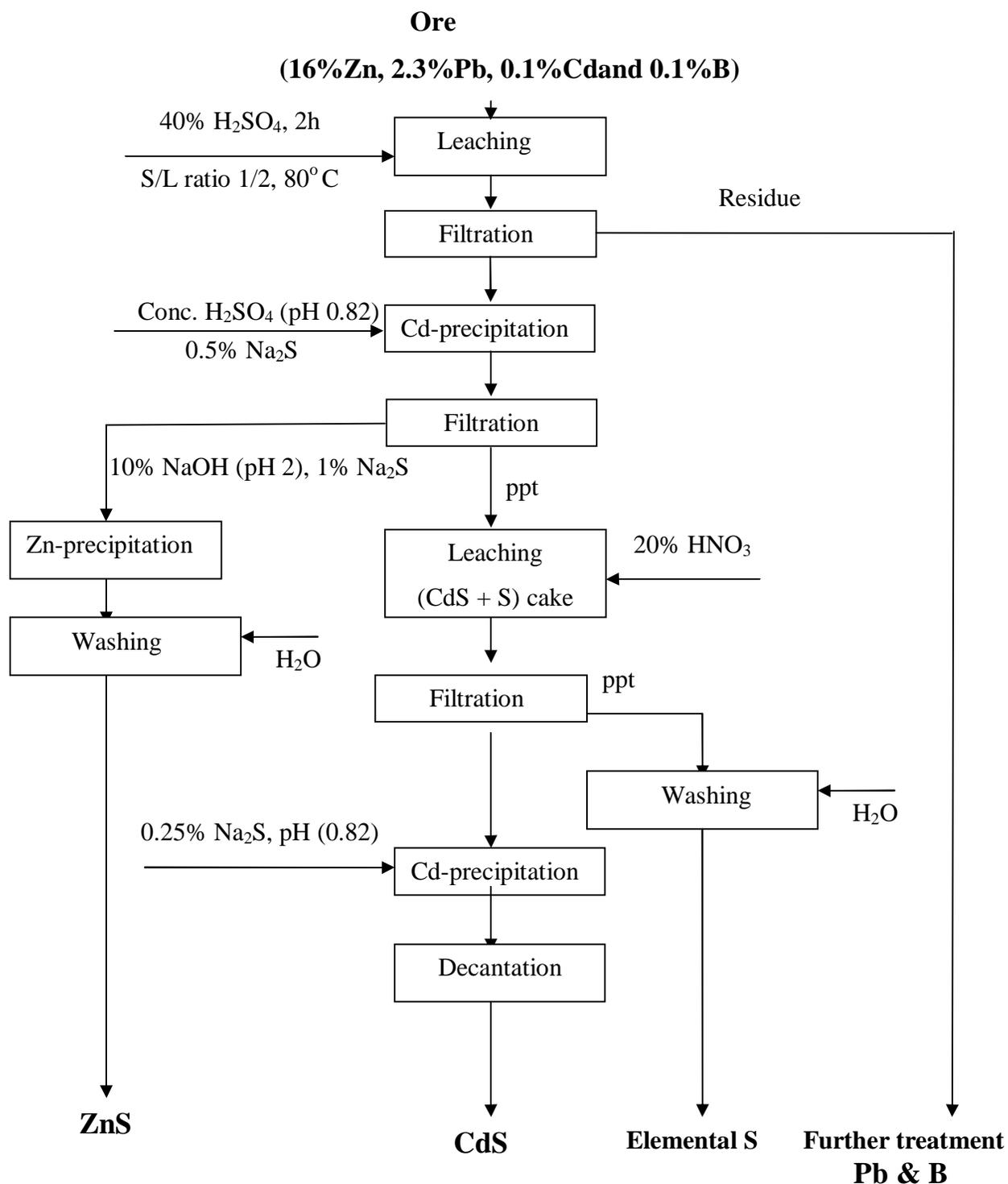
**Figure (4):** A worked flowsheet for separating pure CdS and ZnS from Um-Gheig ore sample
