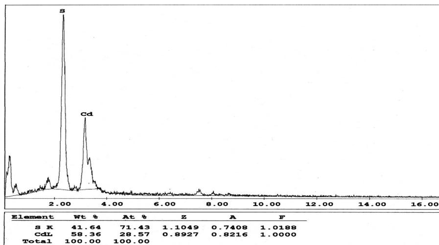
**Figure (2):** EDAX chart for identification of CdS prepared from sulfate leach liquor.
