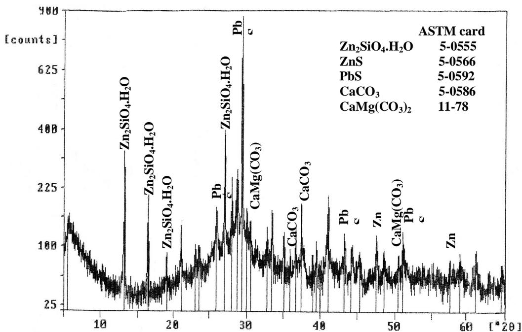
**Figure (1):** XRD chart for the mineralogical study of Um Gheig ore sample
