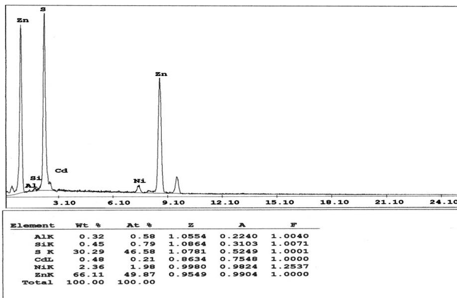
**Figure (3):** EDAX chart for identification of ZnS prepared from sulfate leach liquor.
