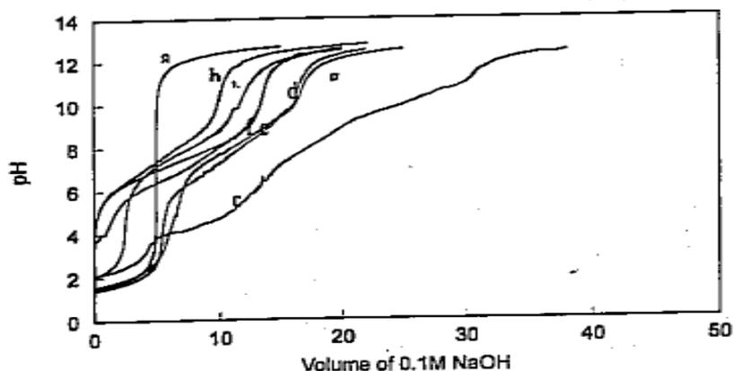
Fig. 1: Potentiometric titration curves of (a) 0.01 M nitric acid, (b) a + 0.02 M levofloxacin, (c) b + 0.01 M Al (III), (d) b + 0.01 M Cr (III), (e) b + 0.01 M Sb (III), (f) b + 0.01 M Bi (III), (g) b + 0.01 M Fe (III) and (h) b + 0.01 M Zr (IV) with 0.01 M sodium hydroxide.
