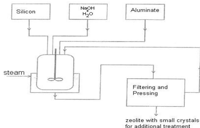
**Figure 2.** Technological Scheme for production of zeolite 4A
