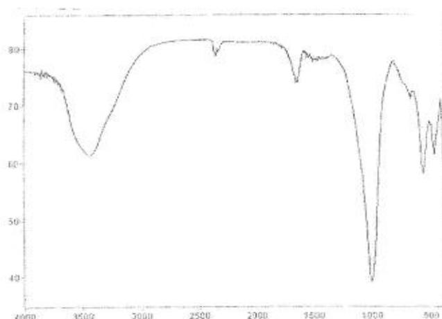
**Figure 5.** IR spectrum of the obtained zeolite from floating ashes
