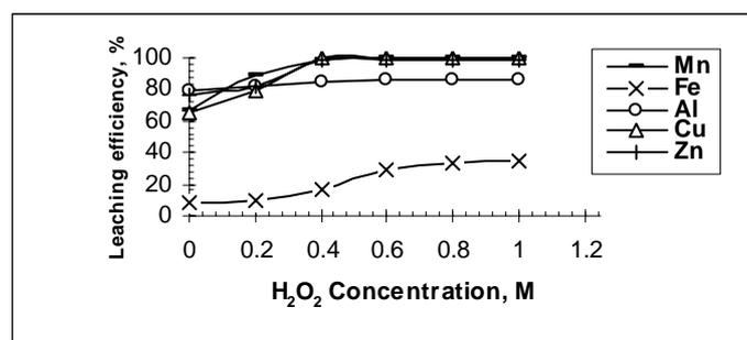
**Fig 2.** Effect of  $\text{H}_2\text{O}_2$  concentration upon the leaching efficiencies of Abu Zeneima studied metal values (2M HCl, 95°C, 1/12 pulp density, 2h, -74 $\mu\text{m}$ )
