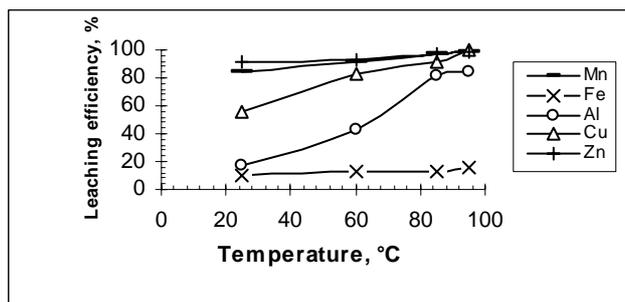
**Fig 3.** Effect of temperature upon the leaching efficiencies of Abu Zeneima studied metal values (2M HCl, 0.4M H<sub>2</sub>O<sub>2</sub>, 2h, 1/12 pulp density, -74 $\mu$ m)
