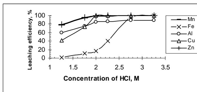
**Fig 1.** Effect of HCl concentration upon the leaching efficiencies of Abu Zeneima studied metal values (0.4M H<sub>2</sub>O<sub>2</sub>, 95°C, 1/12 pulp density, 2h, -74µm)
