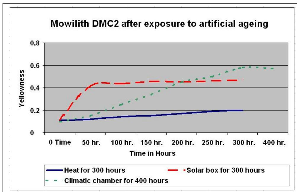
**Fig. 3** Changes in the yellowing rate value of Mowilith DMC2 after exposure to artificial ageing.
