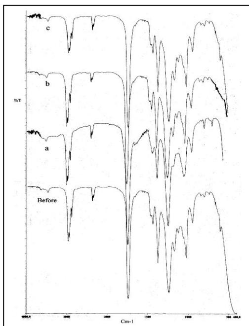
**Fig. 4** FTIR patterns of Mowilith DMC2 before and after exposure to artificial ageing, (a) after exposure to heat, (b) after exposure in solar box, (c) after exposure in climatic chamber.
