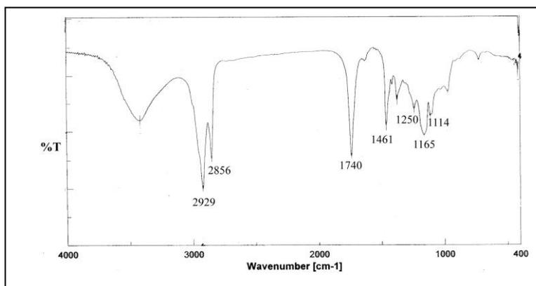
**Fig. 10** FTIR pattern of the linseed oil medium used in the paint layer.
