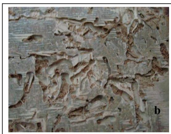
**Fig. 13** The tunnels and insects on the backside of the oil painting that appeared after removal of the first layer of plywood.
