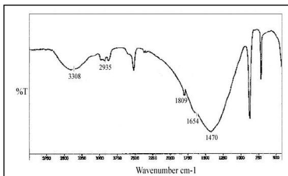
**Fig. 8** FTIR pattern of the glue adhesive in ground layer.
