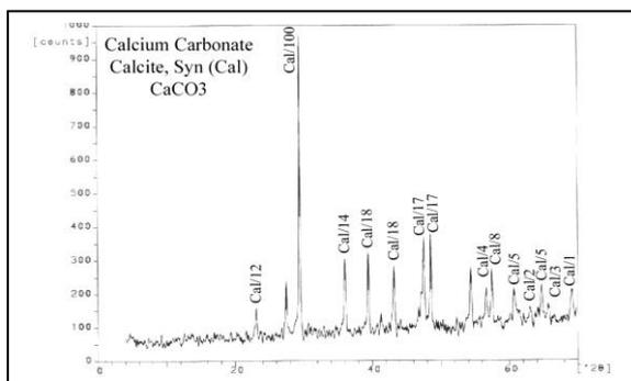
**Fig. 7** XRD Pattern of the ground layer.
