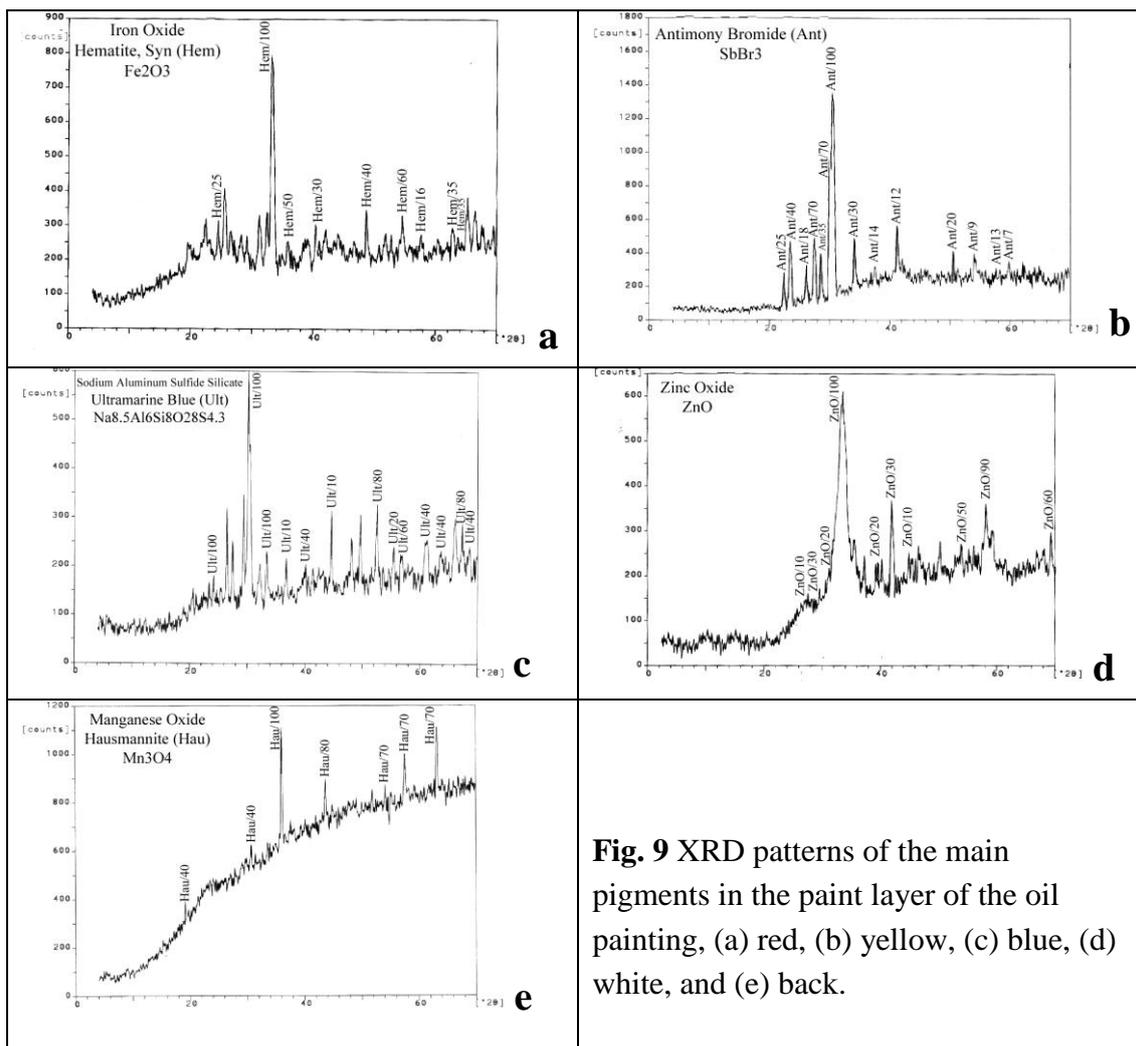
**Fig. 9** XRD patterns of the main pigments in the paint layer of the oil painting, (a) red, (b) yellow, (c) blue, (d) white, and (e) back.
