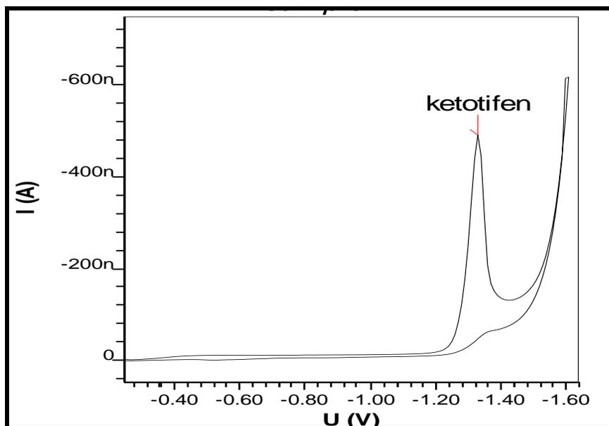
**Fig. 1:** Cyclic voltammogram of  $1 \times 10^{-4} \text{ mol l}^{-1}$  Ketotifen in pH 11 B-R buffer, scan rate  $50 \text{ mV s}^{-1}$ .
