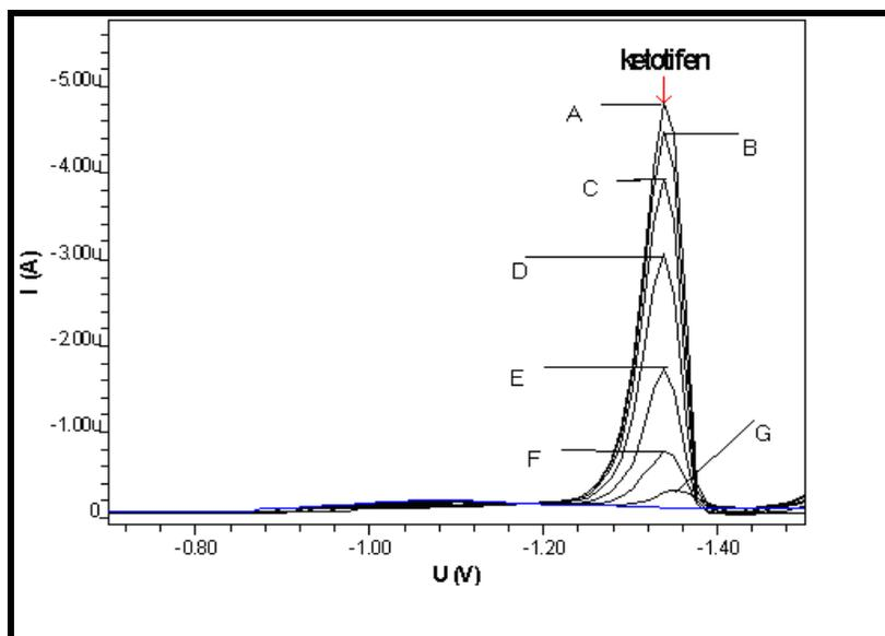
**Fig. 8:** AdSV voltammogram for Ketotifen in B-R buffer (pH 11), pH=11,  $T_{acc} = 90$  sec,  $E_{acc} = -0.60$  V. Drug Conc: (A=  $1 \times 10^{-6}$  M, B=  $8 \times 10^{-7}$  M, C=  $6 \times 10^{-7}$  M, D=  $4 \times 10^{-7}$  M, E=  $2 \times 10^{-7}$  M, F=  $1 \times 10^{-7}$  M, G=  $5 \times 10^{-8}$  M ).
