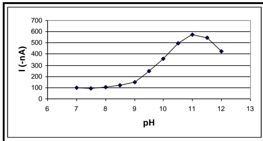
**Fig. 3** Fig 3:..Effect of pH on AdSV peak current.
