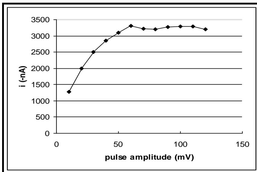
**Fig. 6** Effect of pulse amplitude on AdSV peak current.
