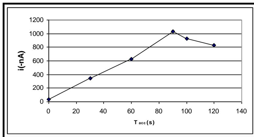
**Fig. 4** Effect of time accumulation on AdSV peak current.
