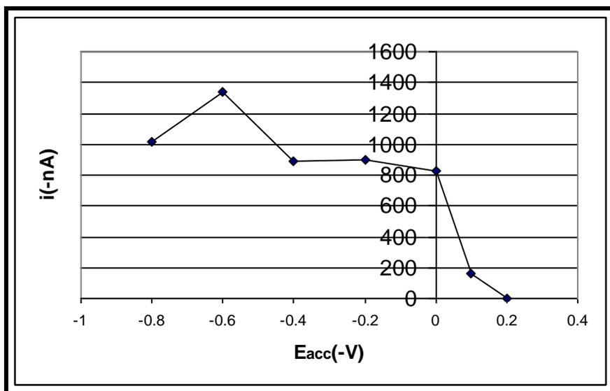
**Fig. 5** Effect of accumulation potential on AdSV peak current.
