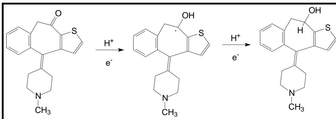
**Scheme1:** the structure and the mechanism of the electrochemical reduction process for ketotifen.
