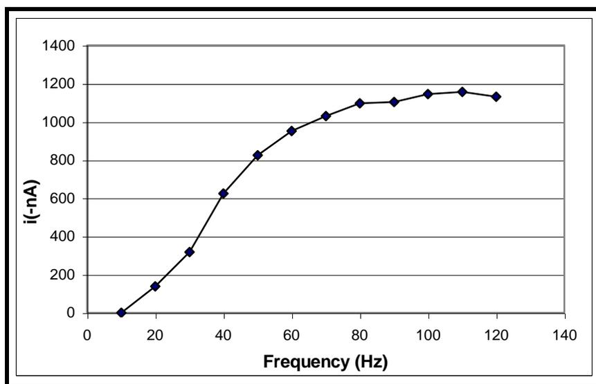
**Fig. 7:** Effect of Frequency on AdSV peak current.
