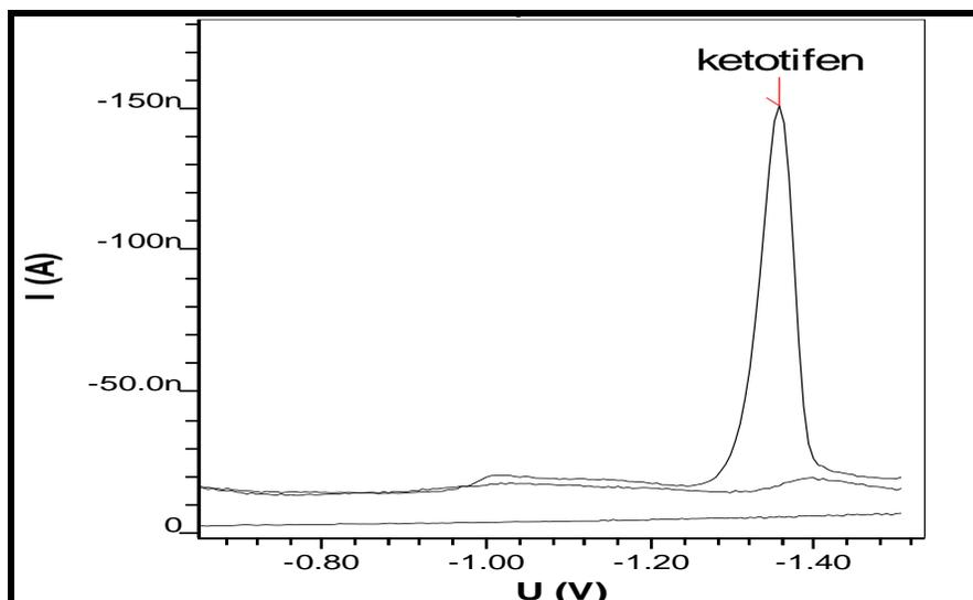
**Fig. 2:** DP AdSV voltammogram of  $5 \times 10^{-7} \text{ mol l}^{-1}$  Ketotifen in pH 11 B-R buffer. Accumulation time 90 sec, accumulation potential  $-0.6 \text{ V}$  and scan rate  $1000 \text{ mV s}^{-1}$ .
