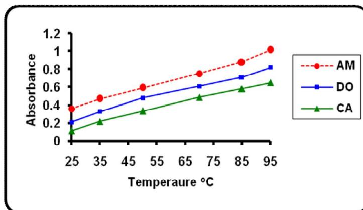
**Fig. 3:** Effect of temperature on the absorbance of AM ( $18 \mu\text{gml}^{-1}$ ), DO ( $6 \mu\text{gml}^{-1}$ ) and CA ( $10 \mu\text{gml}^{-1}$ )-p-DAC (0.5 % w/v) reaction product.
