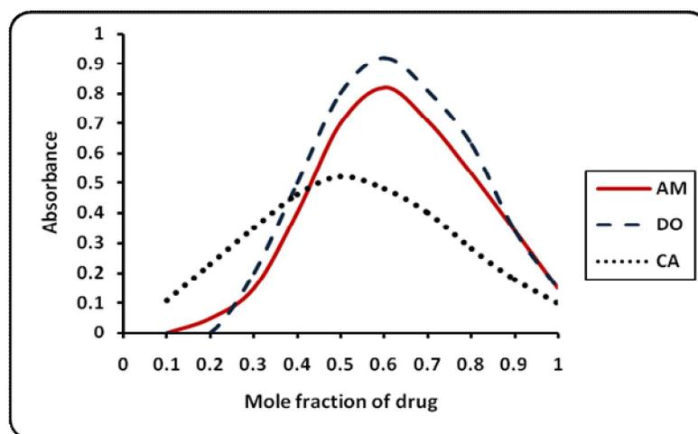
**Fig. 4:** Determination of Stoichiometry of the reaction of amlodipine besylate, dobutamine HCl and carvedilol – p-DAC by continuous variation method using ( $2 \times 10^{-4}$  M) solutions.
