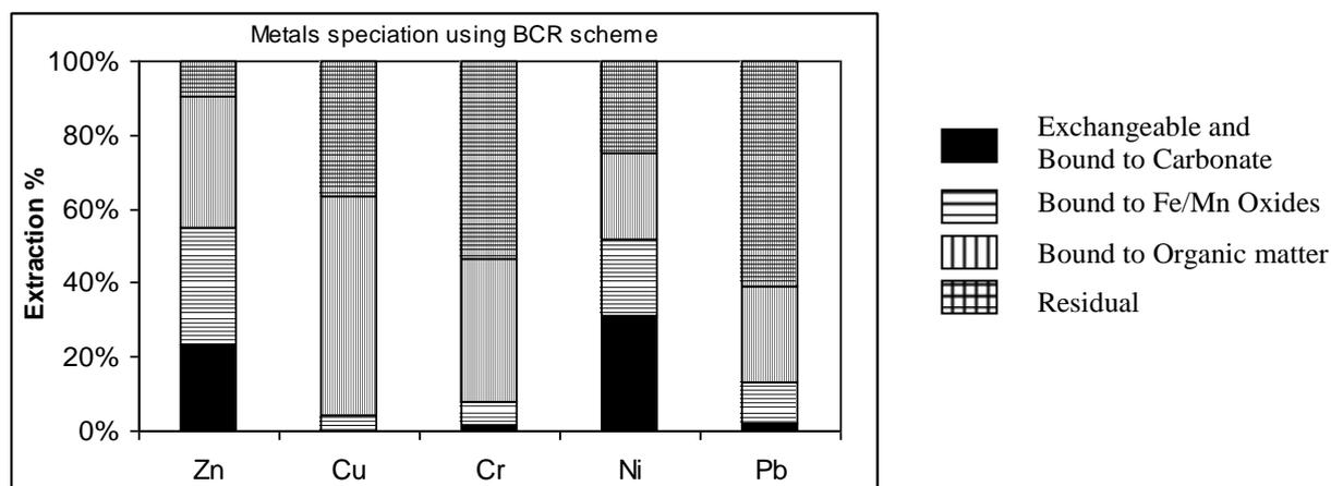
Fig. 2: extraction percentage of metals obtained with sequential extraction using BCR scheme
