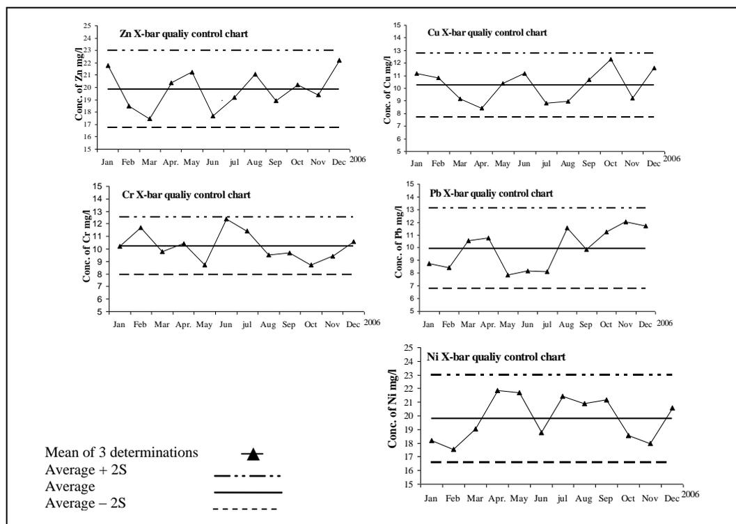
Fig. 3, X-Bar Quality control chart for heavy metals analysis by ICP-OES
