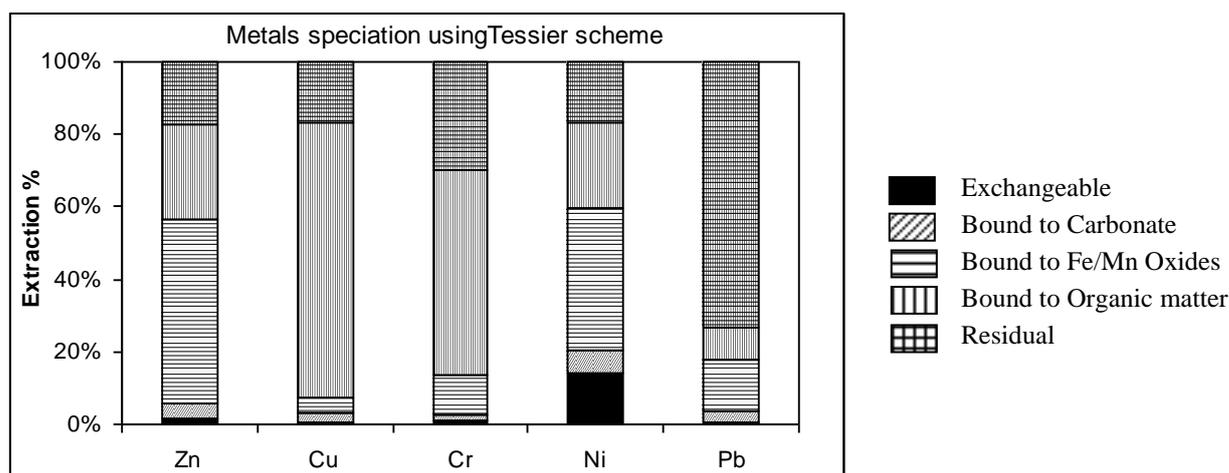
Fig. 1: extraction percentage of metals obtained with sequential Extraction using Tessier's scheme
