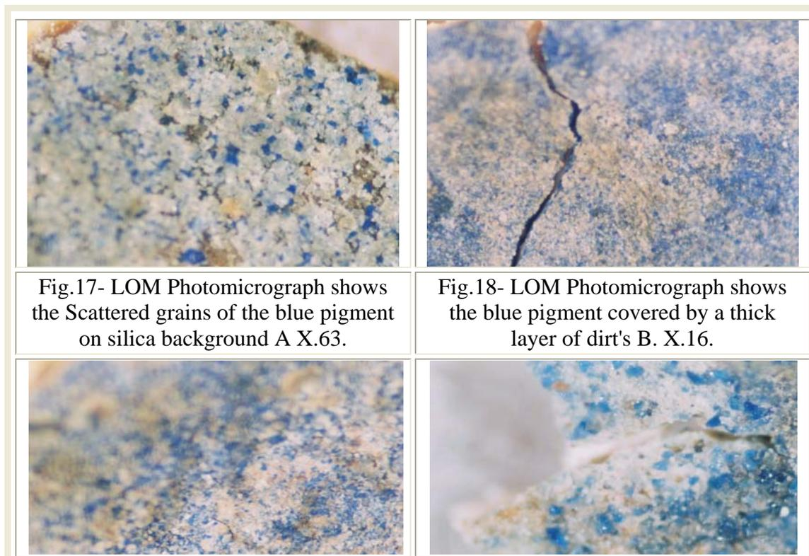
Fig.17- LOM Photomicrograph shows the Scattered grains of the blue pigment on silica background A X.63.
