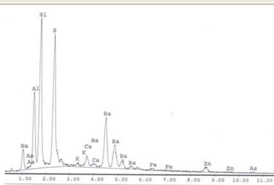
Fig.9 -SEM (EDAX) microanalyses, sample E.
