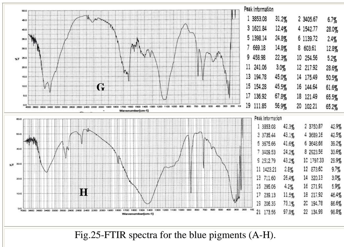
Fig.25-FTIR spectra for the blue pigments (A-H).
