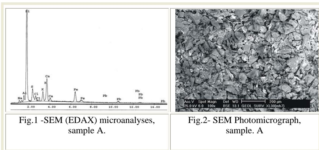
Fig.1 -SEM (EDAX) microanalyses, sample A.
