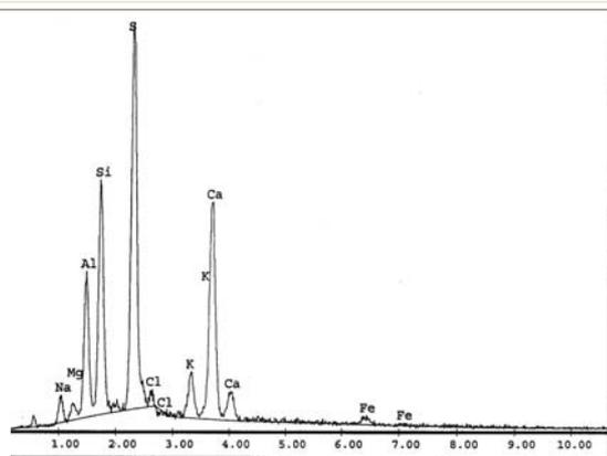
Fig.13 -SEM (EDAX) microanalyses, sample G.
