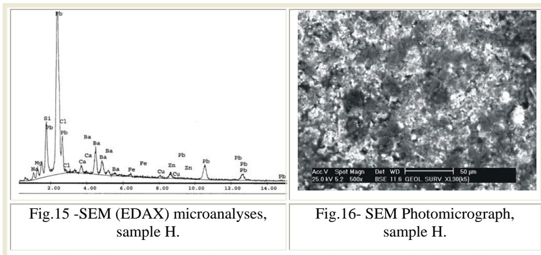
Fig.15 -SEM (EDAX) microanalyses, sample H.
