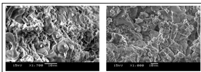
**Fig (4)** Shows voids due to lose of binding material and salts crystallization between
